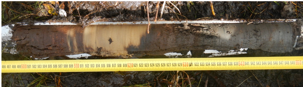
Figure 3: LRC4 core. The LRC4 peat core shows clear stratigraphic changes, from clayey inorganics (gray) to peat (brown), to sandy materials (beige), and back to peat (brown). Photo credit: Daniel Karran
