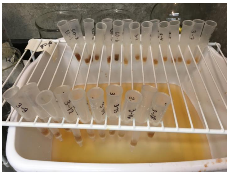
Figure 4. Cellulose Extraction. Image of whole wood samples being drained of sodium hydroxide solution prior to being washed with distilled water.
