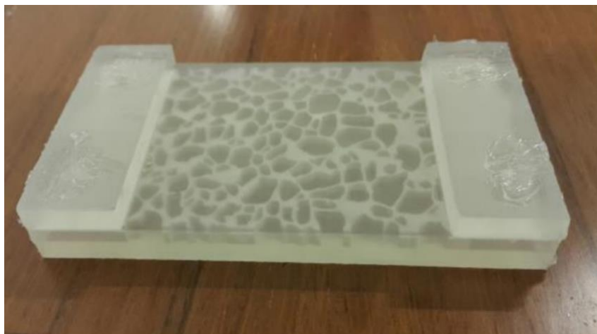
Figure 5. 3D printed micro-model using transparent resin (an example of heterogenous porous media).
