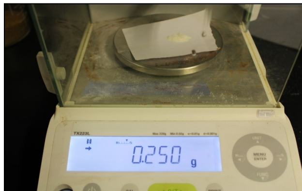
Figure 18: Weighing the 0.1 wt% Flowzan.
