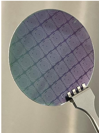
Figure 7: Correctly exposed photoresist pattern
