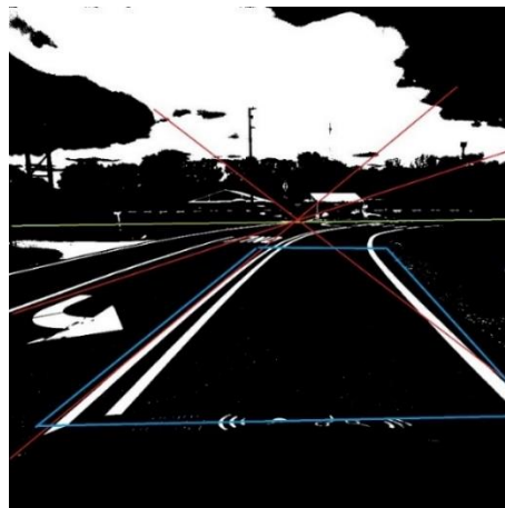
Fig. 2.7 Vanishing Point for Curved Lane Detection Green line is the Vanishing Point Line, Red lines are all lane edges present in the environment, Blue Box show the Region of Interest
