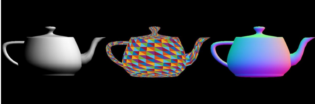
Figure 1.1: The left teapot is lit using rasterized lighting. The middle teapot illustrates the triangles used to describe the teapot. The right teapot is a rasterized view of the normal of the model.
