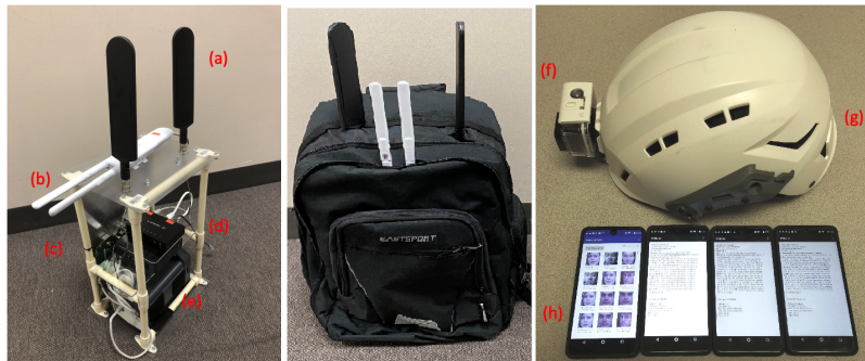
Figure 2.2: DistressNet-NG - a MEC platform for disaster response consisting of: a) LTE antenna, b) Wi-Fi AP, c) LTE eNB, d) Intel NUC that runs LTE EPC and HPC; e) Battery; f-g) Helmet with body camera; h) Android phones
