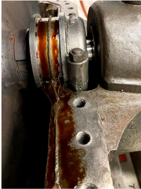
Figure 4.5 Application of Temp Tight II on the bottom part of the casing.
