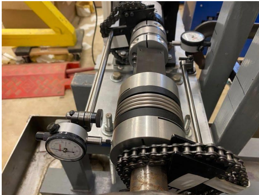
Figure 4.13. Horizontal misalignment setup.
