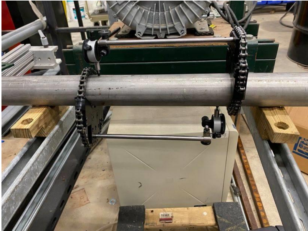
Figure 4.12. Bar sag measurement setup.
