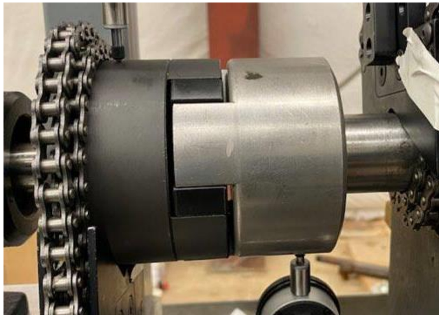
Figure 4.8 Lovejoy L110 rubber spider coupling mounted between the turbine and the dyno.
