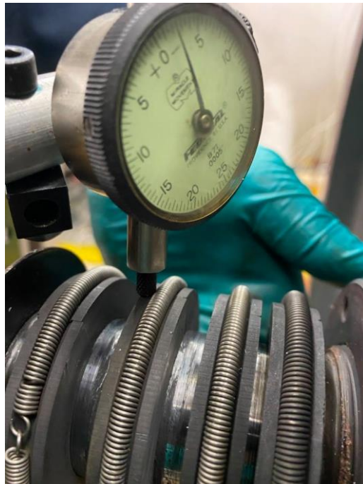
Figure 4.2 Sealant quality check. The dial gauge reads less than 5 mils, which is the clearance between the shaft outer surface and the carbon inner surface.
