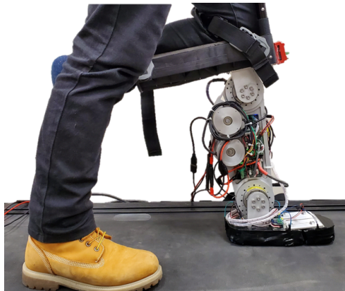
Figure 3.2: AMPRO II—a transfemoral prosthesis attached to a L-shaped emulator
