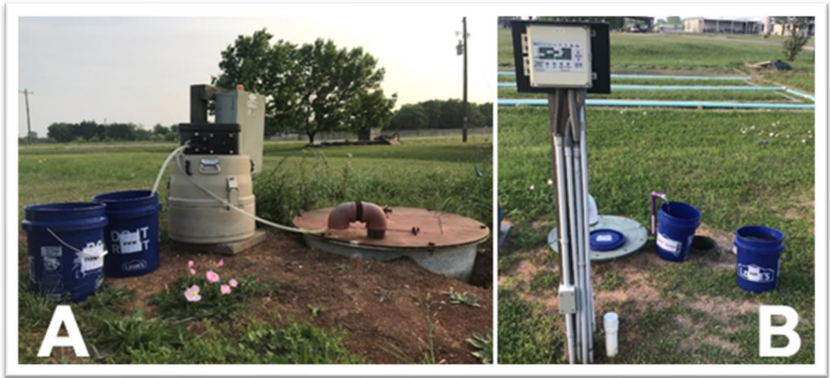
Figure 2.2 A) Taking water from the raw wastewater tank through ISCO 3700, B) Taking water from the MBR treatment system (B)
