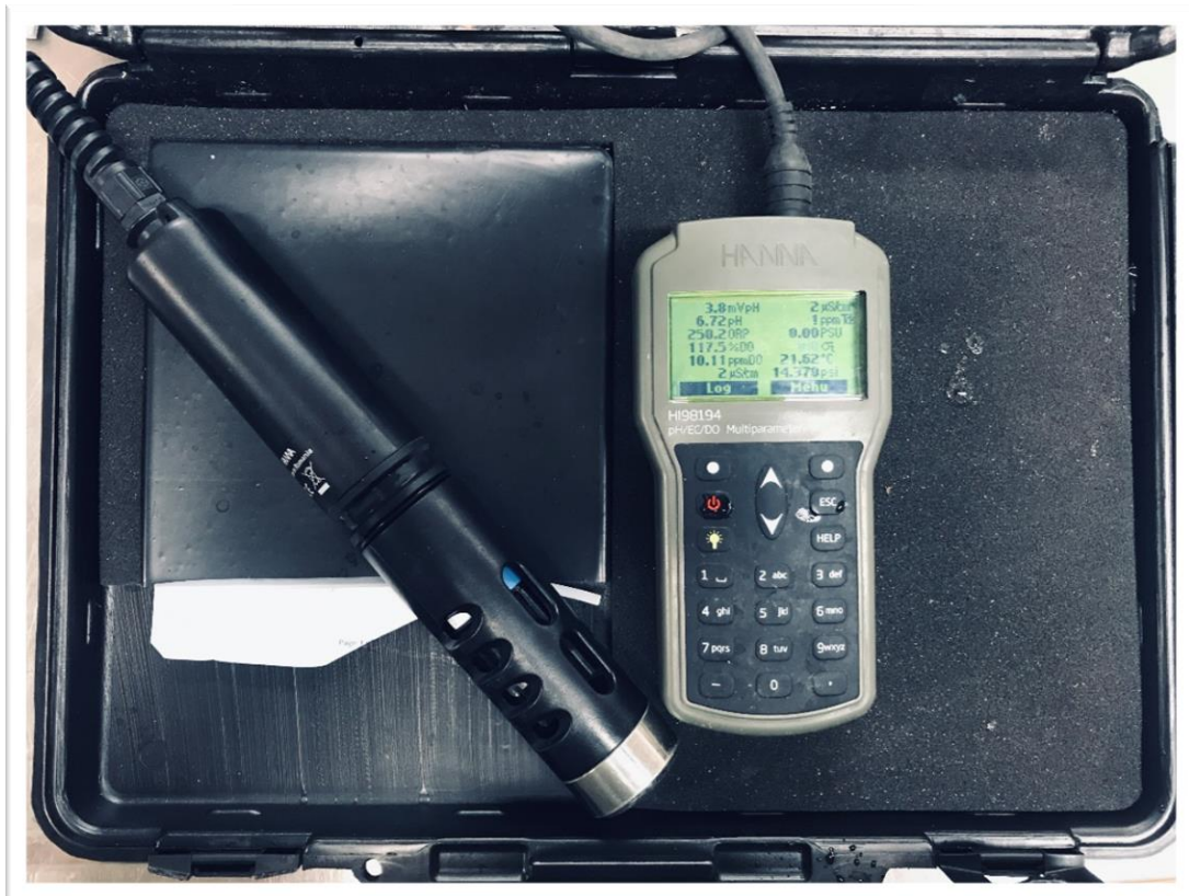
Figure D.4 Hanna HI98194 Multiparameter Meter
