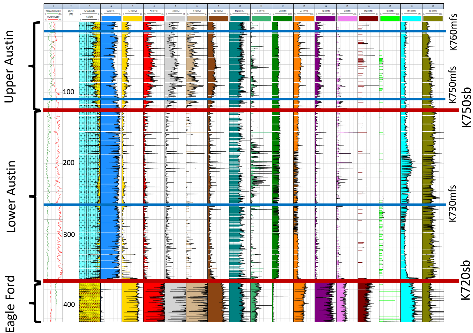
Figure 8. Elemental distribution of cored Well-X section by element using the Bruker Tracer 5i. Sequence boundaries and maximum flooding surfaces marked with red and blue lines respectively. Upper and Lower Austin Formations marked.
