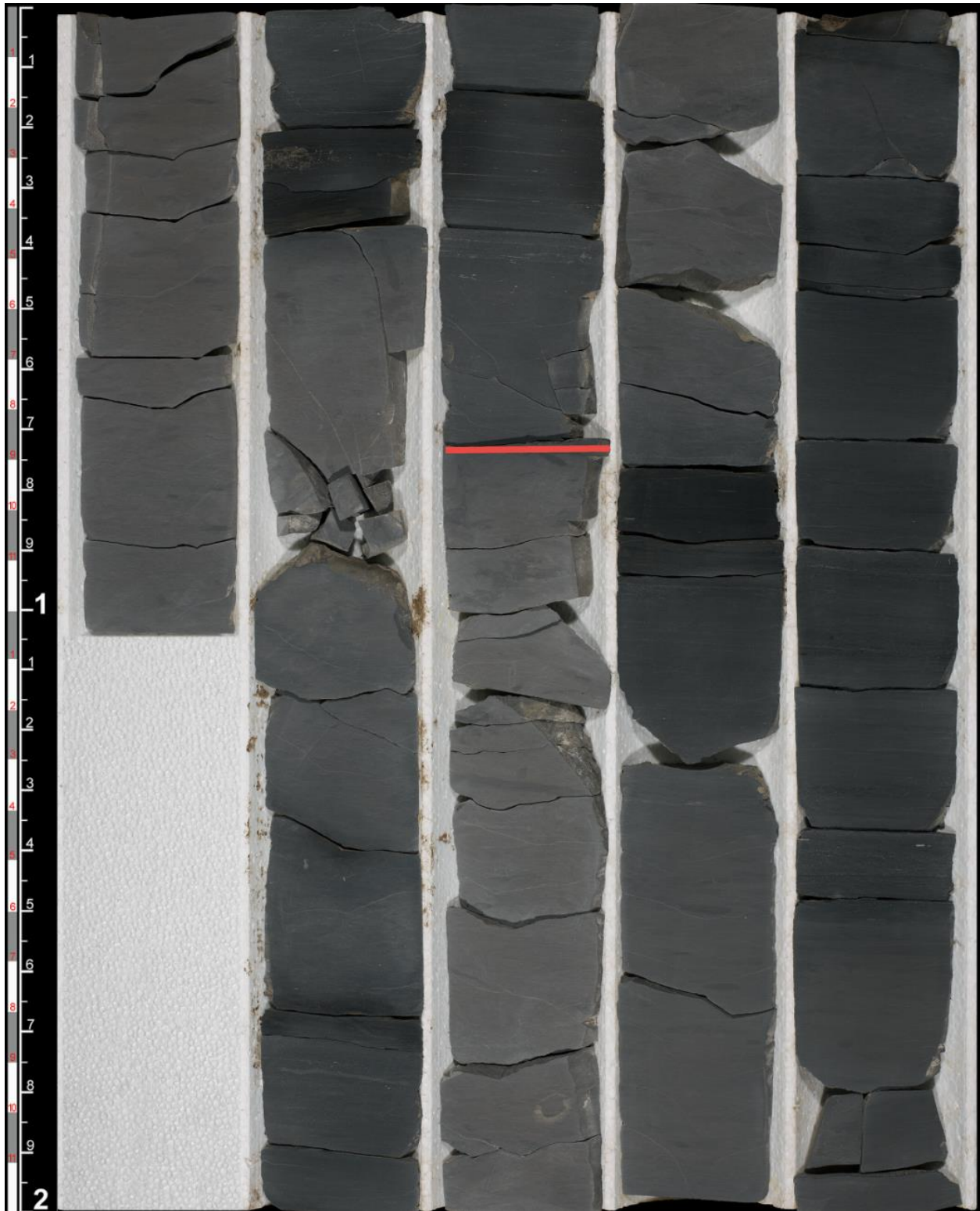
Figure A16. Core photo of the Upper and Lower Austin boundary (K750sb). Boundary marked in red.
