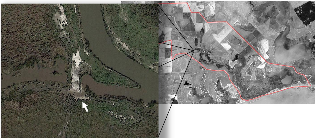
Figure 16. Barrier to flow on Big Boggy Creek. This structure (barrier 1 in Table 2 & Figure 15) does not appear to have culverts and instead allows the water to flow over the top.
