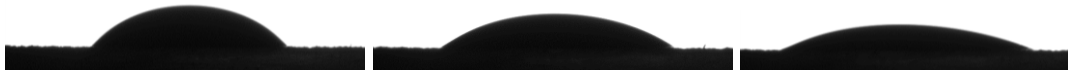
Figure 4.4: The three contact angle measurements of the same droplet, with 3-minute time intervals.
