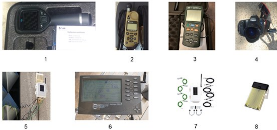
Figure 3.10: Equipment for measurement campaign for 2019 and 2020. 1-FLIR E6 thermal imaging camera, 2- Kestrel 2400 Heat Stress Tracker, 3 – Solar Meter, 4- Canon EOS fisheye camera, 5- Davis weather station, 6- Davis Vantage Pro 2, 7 – soil moisture and temperature probes, 8 – leaf temperature and wetness sensor.
