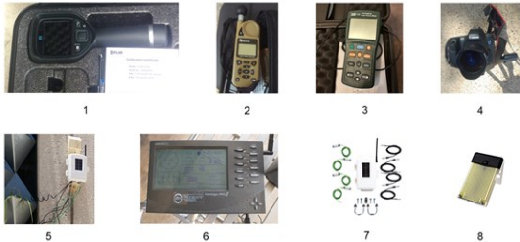
Figure 1.4 Equipment for measurement campaign for 2019 and 2020. 1-FLIR E6 thermal imaging camera, 2- Kestrel 2400 Heat Stress Tracker, 3 – Solar Meter, 4- Canon EOS fisheye camera, 5- Davis weather station, 6- Davis Vantage Pro 2, 7 – soil moisture and temperature probes, 8 – leaf temperature and wetness sensor.
