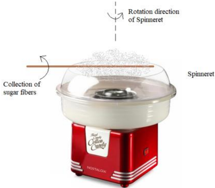
Figure 2.1 Preparation and collection of sugar fibers using a countertop cotton candy maker
