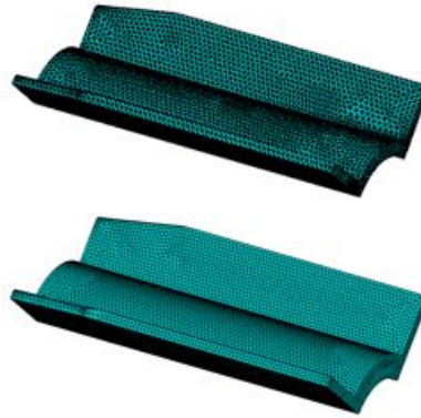
Figure 3.9: Meshes for convergence study, 2mm (top) and 1.5 mm (bottom) max node spacing.
