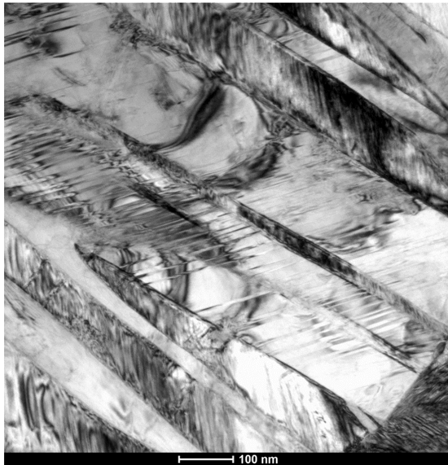
Figure 2.1: Representative TEM micrograph of Ti-rich Ni-Ti-Hf alloy aged at 550 °C for 3 h and air cooled. The alloy does not show any precipitates formed in the martensite matrix [6].
