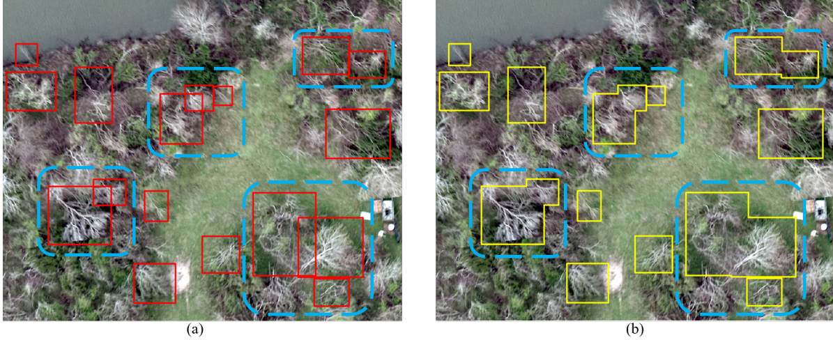
Figure 5.9: Example of creating clusters based on overlapped fallen trees. Red rectangles represent the original polygons, and yellow rectangles denote merged polygons. Merged bounding boxes are highlighted in blue rectangles
