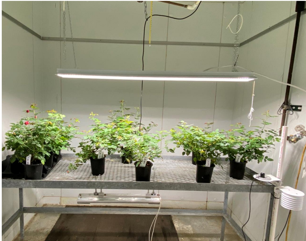
Figure 4 Heat chamber with heater under the bench of plants and light and humidity sensors.
