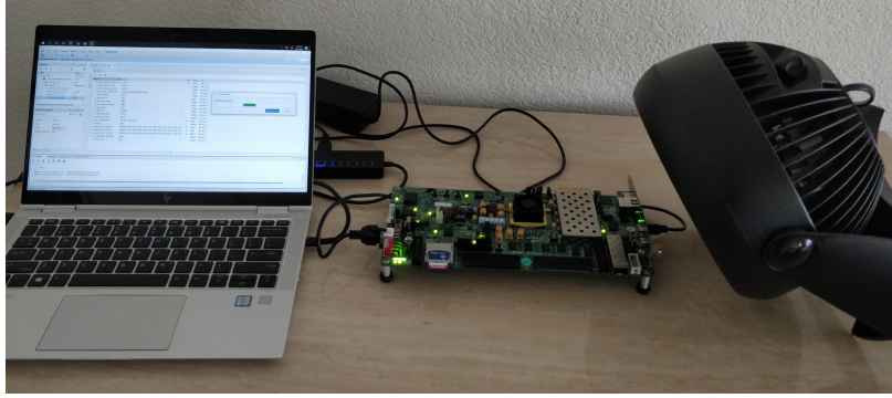
Figure 4.5: All experiments in this work are demonstrated on the Zynq ZC706 FPGA evaluation platform. The board is connected to the host machine, where the power traces are collected to perform correlation power analysis (CPA) attacks. Apart from the fan on the heat sink to reduce the FPGA junction temperature, we also placed a table fan to cool the FPGA board further.
