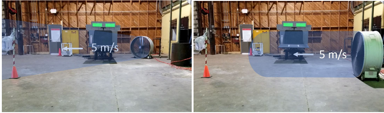
(a) Diagonal wind testing setup
