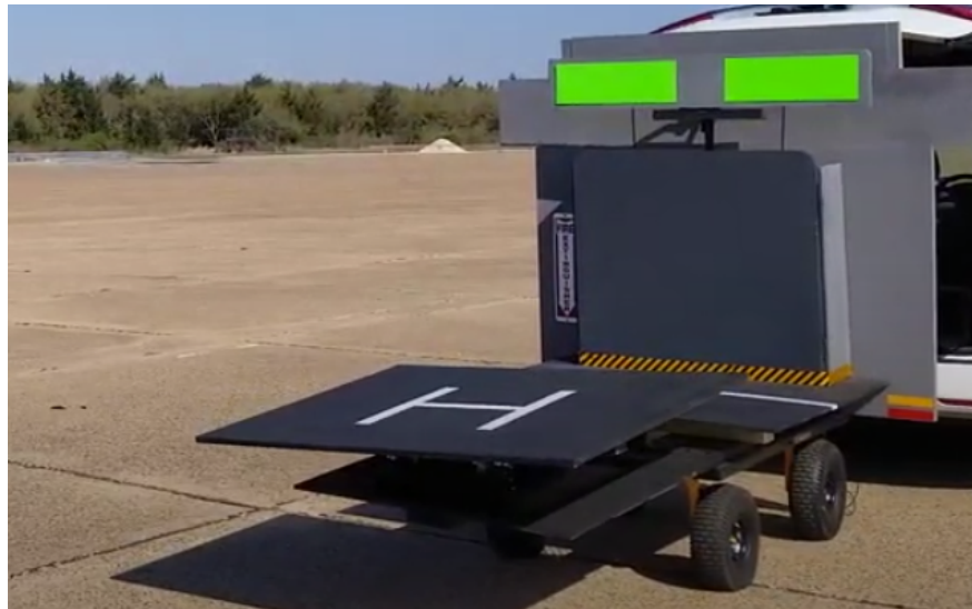
Figure 4.3: Constructed ship platform with horizon bar and motion deck [2] [3]
