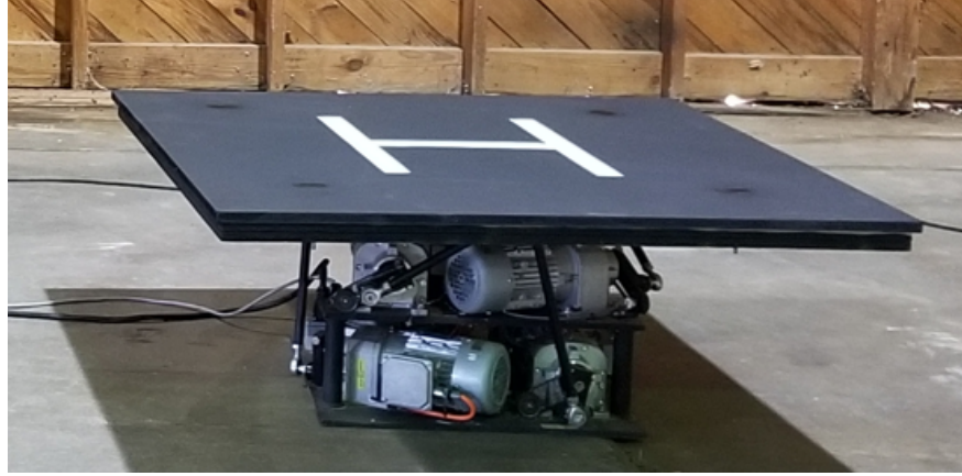
Figure 4.2: Servos and Simulation Inc. 6 DOF motion system with 1.22 x 1.22 meters(4 x 4 feet) Landing Deck [2] [3]
