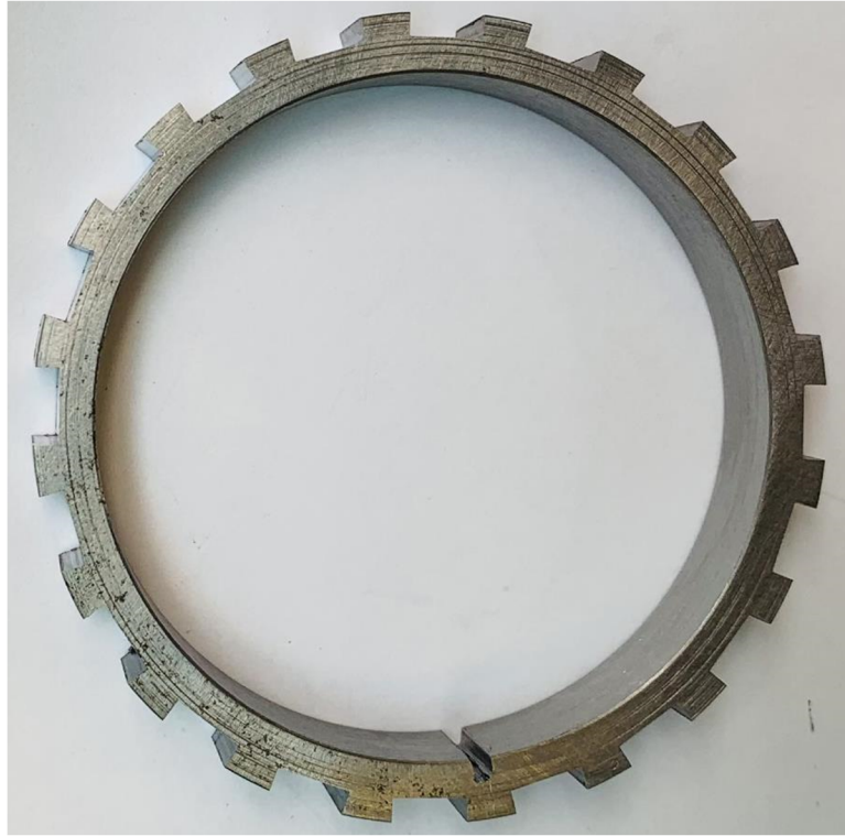
Figure 7.2: The (a) PMs and (b) back iron of the inner rotor in the CP CyMG prototype.
