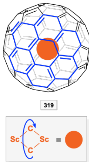
Figure 2.68 Solid endohedral fullerene C_2Sc_2@C_{84} ( 319 ), considered an example of a quantum gyroscope.
