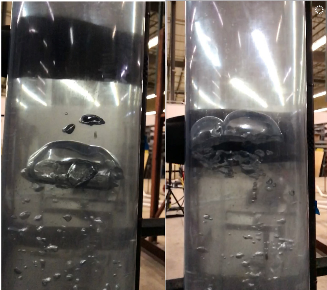
Figure 2-6—Gas bubble expansion experiments under vacuum conditions. Reprinted from (Kaldirim and Schubert 2018)
