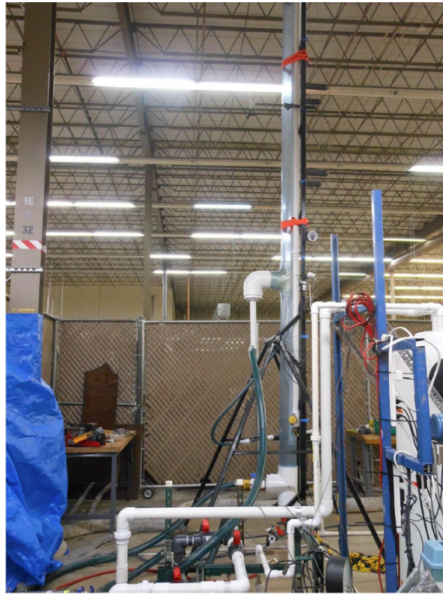
Figure 2-1—DGD Lab Riser Model at 0° from Vertical Reprinted from (Kaldirim 2015)
