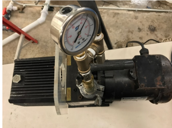
Figure 2-4 —Vacuum pump used in experiments. Reprinted from (Kaldirim and Schubert 2018)
