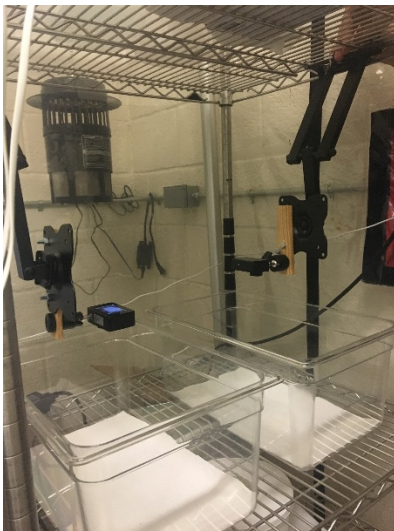
Figure 1: Experiment arena with polycarbonate containers lined with white bench paper and Yi Lite cameras docked above
