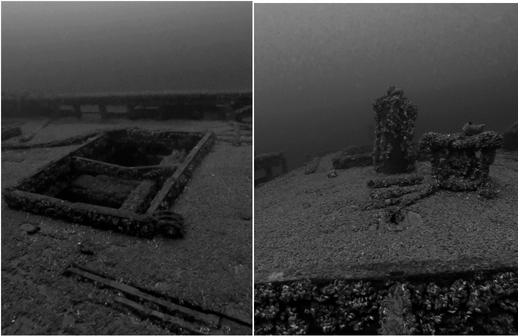
Figure 12. (Left) The centerboard visible at the midships hatch. (Right) The centerboard pennant hole and chain looking aft (© Institute of Nautical Archaeology/ Author, 2021).
