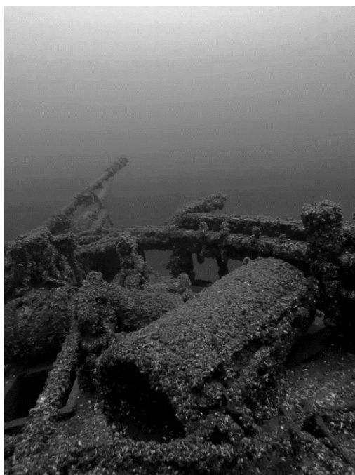
Figure 22. (Left) The vertical boiler resting on the fore deck. (Right) the hoisting winch set forward of the fore hatch (by Author, 2019).
