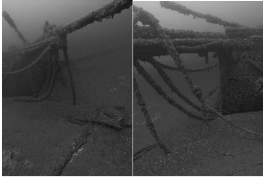
Figure 19. (Left) The bowsprit and jib boom with the bobstays, starboard and port bowsprit guys, jumbo jib stay, and jumbo jib boom. (Right) Portside view of the bowsprit (Photo by Author).
