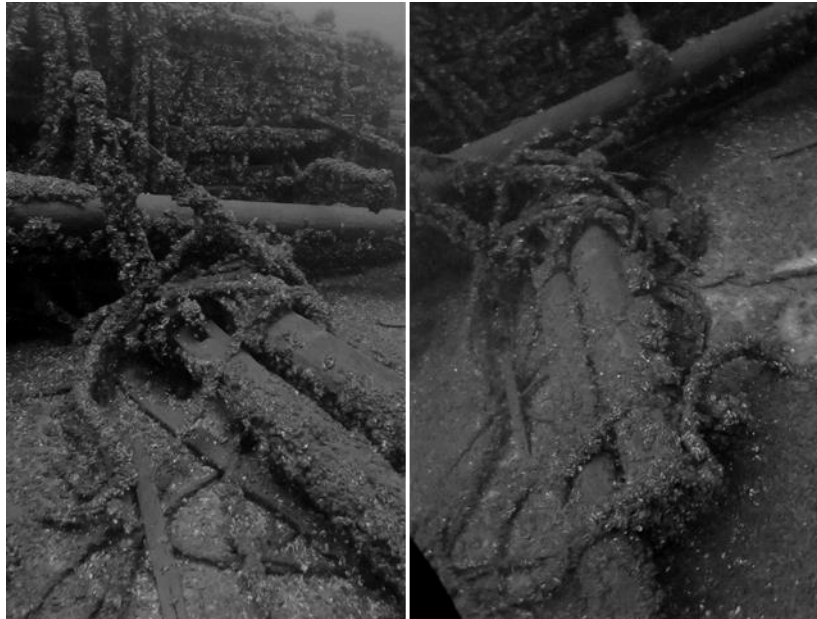
Figure 20. The foremast doubling with the topmast fid and the remains of the crosstrees visible.
