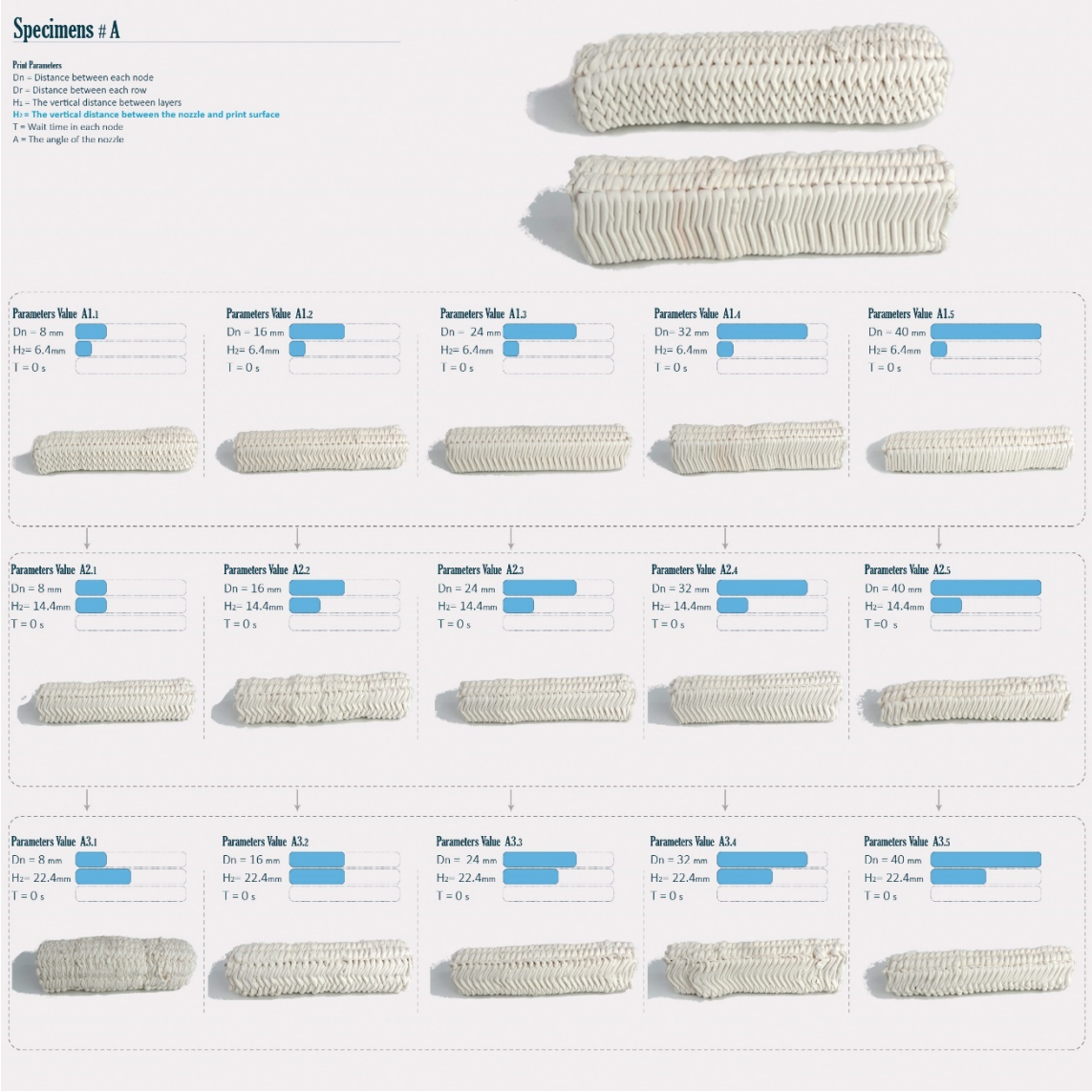
Figure 2.12: The proposed pattern library to be used by an architect or an AI algorithm based on architectural forms and structural requirements
