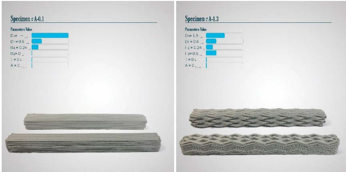
Figure 2.8: Physical specimens printed at the lab before the 3D reconstruction step
