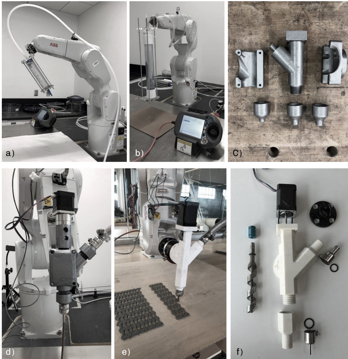
Figure 1.3: Several iterations were developed and tested in order to create an optimal extruder for depositing the novel material supplied by the research group
