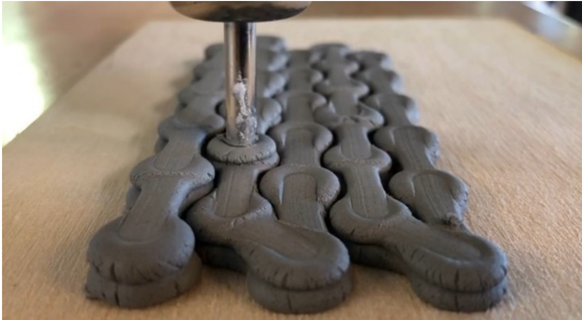
Figure 3.4: Increased material deposition at the stopping points theoretically enhances the surface contact between successive layers
