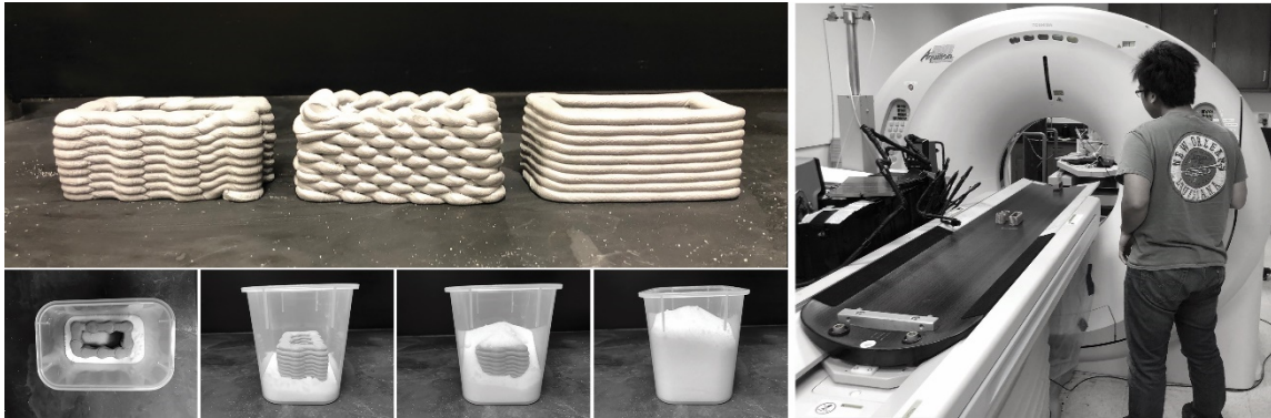
Figure 2.9: Preparing specimens for X-ray CT scanning. As a granular material, table sugar facilitated the transition from a low-density environment into a dense one to increase the accuracy of the scan
