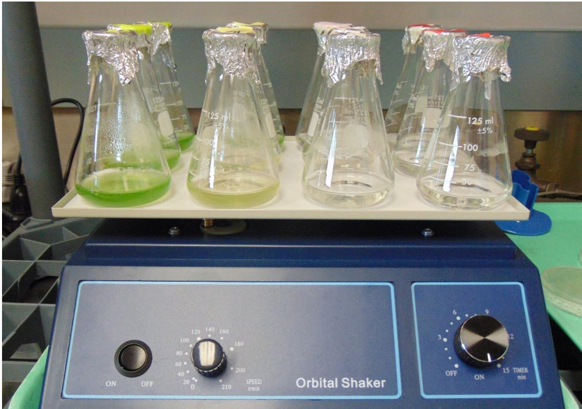
Figure 7. Irradiated cultures exhibited a visibly detectable color change over time following irradiation. From left to right: 0, 0.6, 2.1, and 4.9 kGy.
