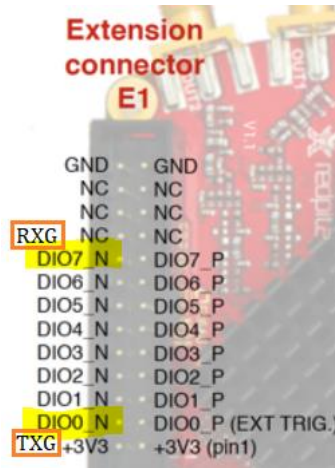
Figure 8: TXG and RXG connections on E1 of Pitaya – highlighted. Modified from Extension — Red Pitaya 0.97 documentation [41]
