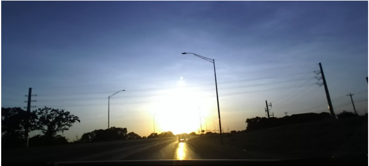
Figure 1.4: RGB camera hindered by direct sunlight, taken with a ZED camera. Reprinted with permission from [29]. ©SAE International.
