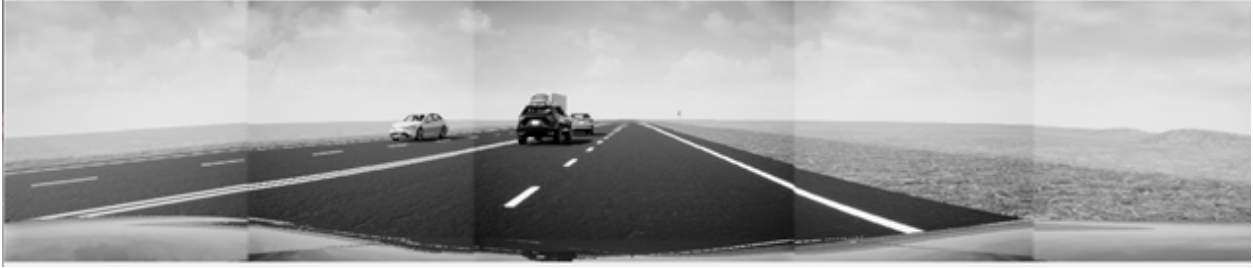
Figure 8.1: A screenshot showing stitched video, as seen through simulated cameras, from the ego vehicle.
