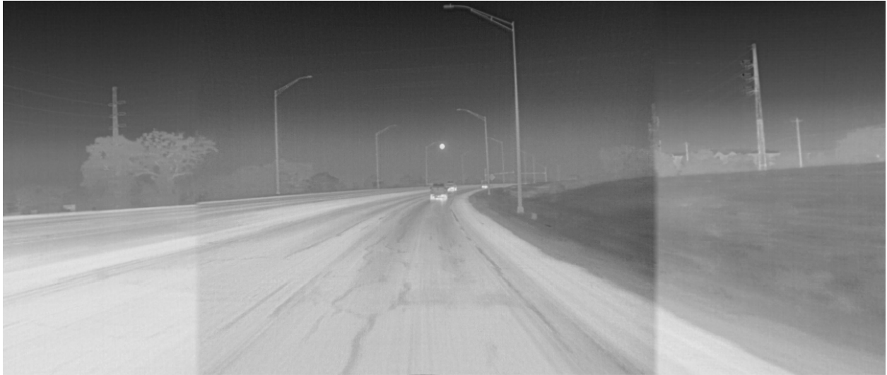
Figure 1.5: Thermal cameras are resilient to direct sunlight. Reprinted with permission from [29]. ©SAE International.
