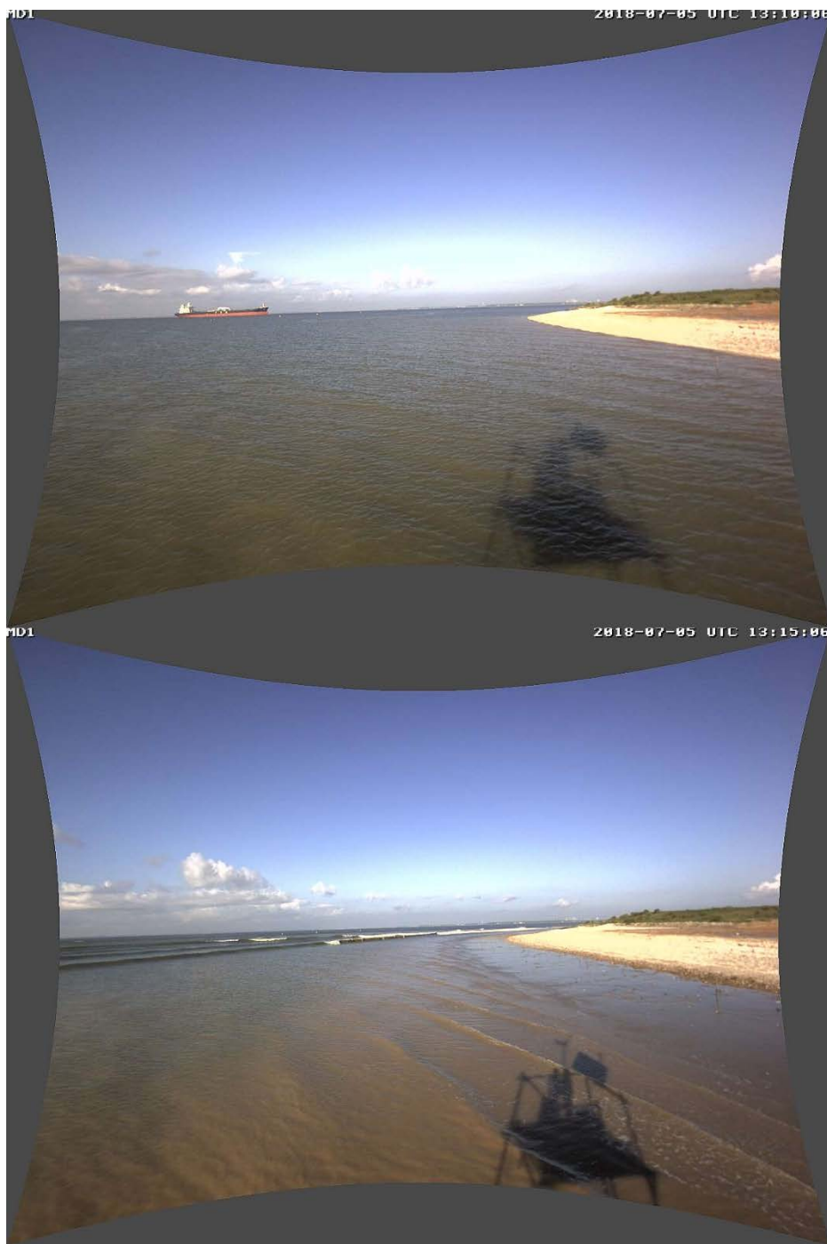
Fig. 4 – Before and after a 140.5-second long, 0.55-meter Bernoulli wave drawdown caused by inbound tanker “ALASKA” (seen in the top image). Bottom image taken 5 minutes after the top and illustrates the maximum extent of the drawdown magnitude as well as the arrival of the leading Havelock surface wave marking the onset of the return surge.
