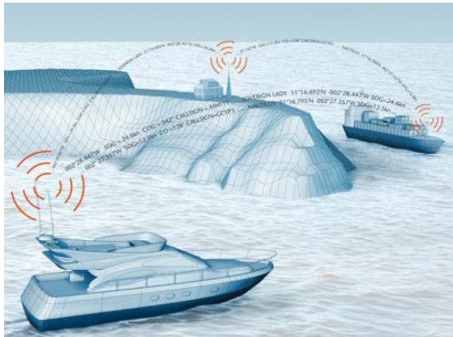
Fig. 19 – Cartoon schematic detailing the principles of AIS. Marine traffic control information can be observed passing between the vessels and shore-based station. Image adapted from IMO (2019).
