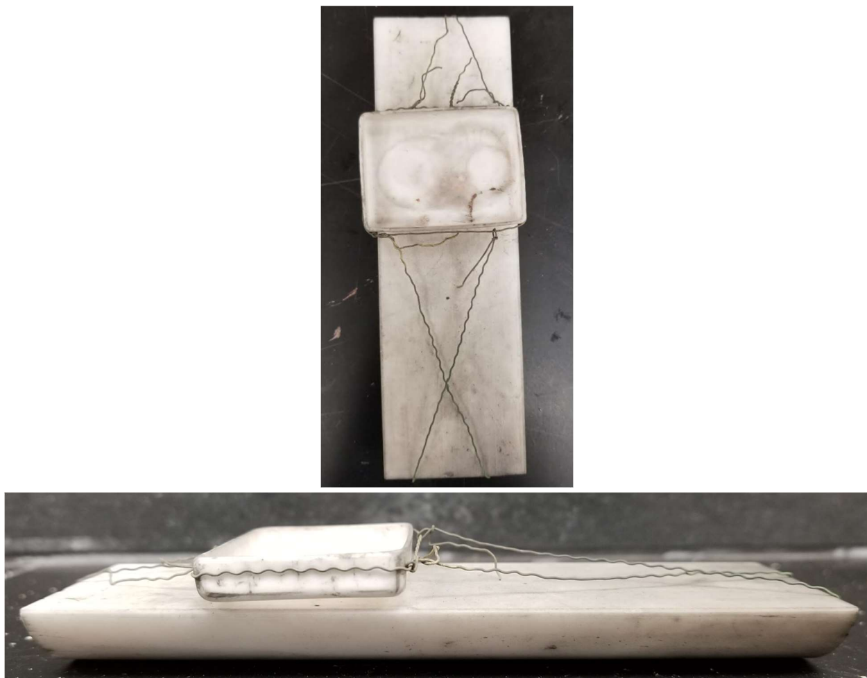
Figure 15: Sample tray placed on set location on top of the dee-tube, held in place by tungsten wire to prevent shifting of loose packed powder during handling or sintering.
