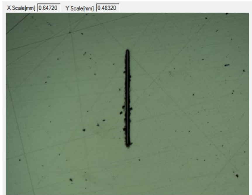
Figure 78: Optical image of nanoscratch on surface of Co-Cr-Mo sample.
