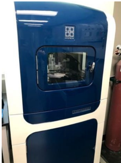
Figure 37: Hystiron TI-950 Triboindenter nanomechanical test apparatus.
