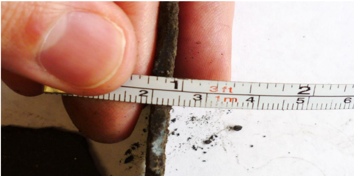
Figure 10.-Thickness of the layer obtained using Eagle Ford cuttings and 500 psi closure stress
