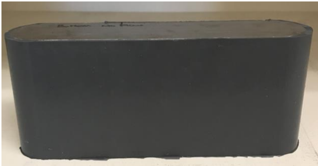
Figure 4.-Steel plate sample assembly covered in rubber epoxy and ready for testing
