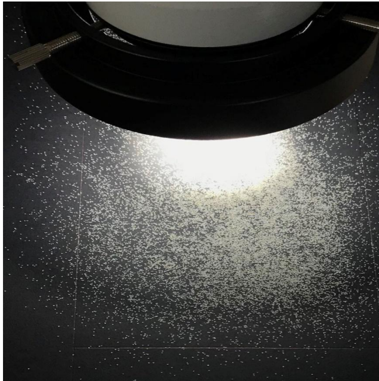
Figure 50.-Proppant sample spread on a black surface paper
