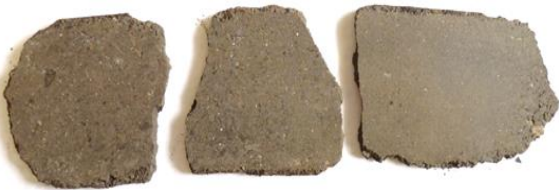
Figure 9.-Layer obtained using Eagle Ford wet cuttings and 500 psi closure stress
