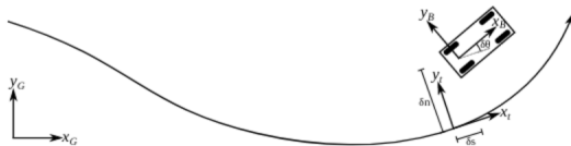
Figure 3.2: The three types of path following errors (a) cross track error ( \delta n ) (b) along track error ( \delta s ) (c) heading error ( \delta \theta )
