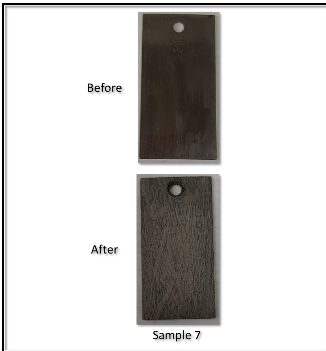
Figure 21: Pictures of N-80 coupon before and after corrosion test with 2 wt.% of sample 7 at 250°F in 15 wt.% HCl and 1 wt.% of each corrosion inhibitor intensifier for 6h.
