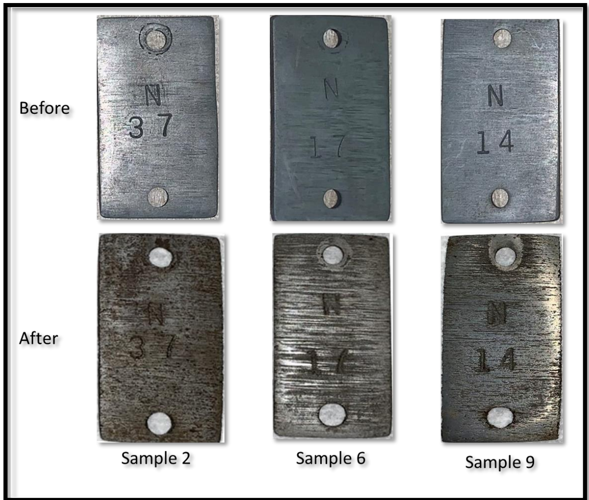
Figure 15: Pictures of N-80 coupons before and after the corrosion test at 150°F in 15 wt.% HCl for 6h for samples 2, 6, and 9. These coupons did not pass the corrosion test.
