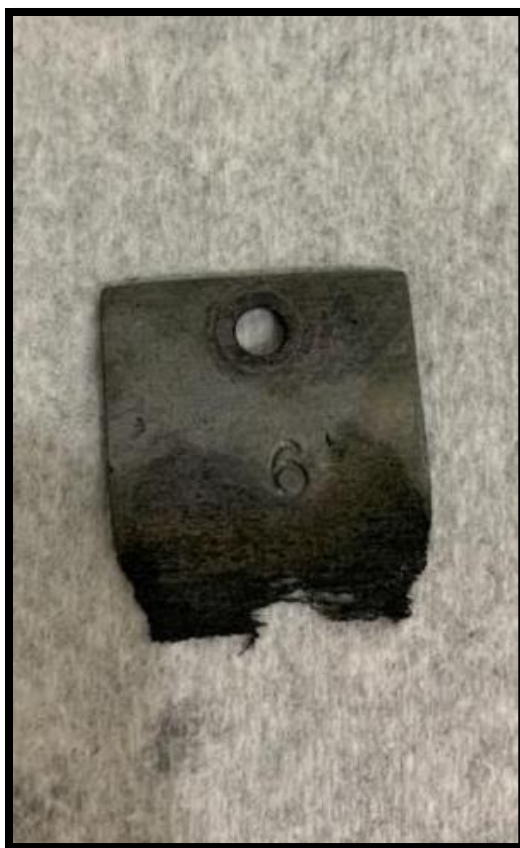
Figure 29: Coupon obtained after testing with anionic emulsifier at 250°F. Half the coupon was dissolved.
