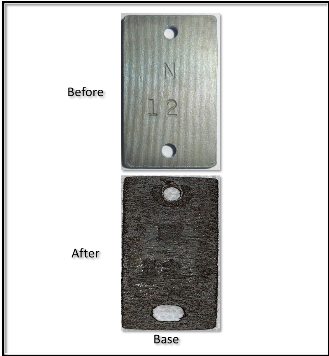
Figure 17: Pictures of N-80 coupon before and after corrosion test at 200°F in 15 wt.% HCl and 2 wt.% corrosion inhibitor intensifier for 6h.
