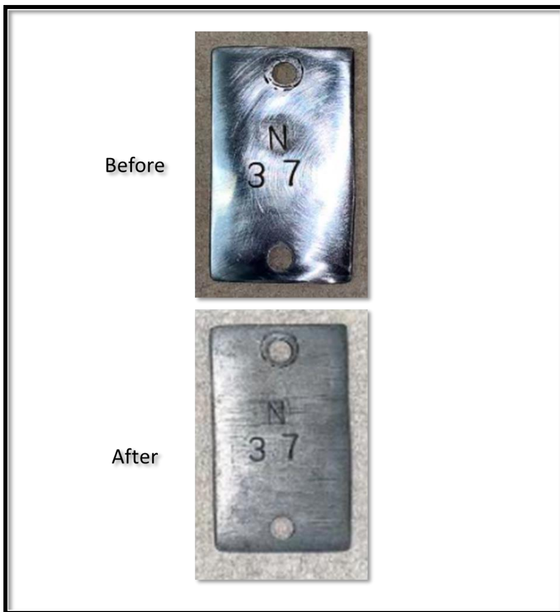
Figure 55: Before and after images of N-80 coupon after the corrosion test with melatonin in 15 wt.% HCl at 150°F for 6h.
