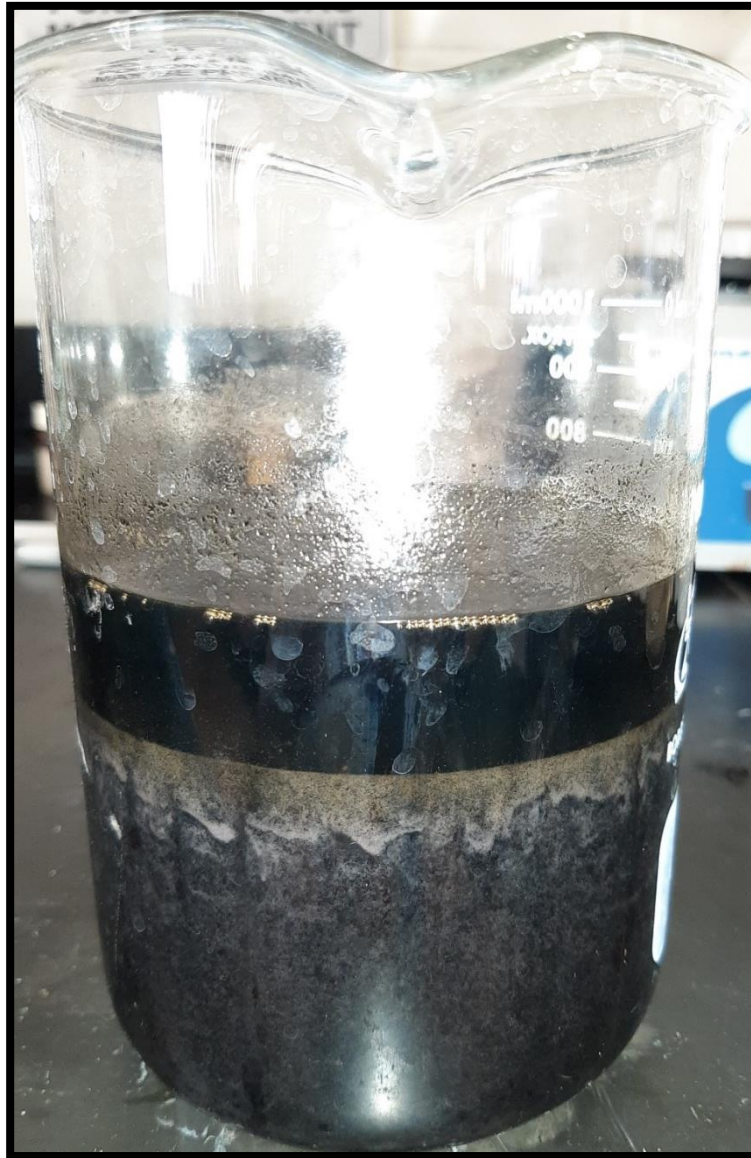
Figure 30: Broken emulsified acid after 250°F test. Anionic emulsifier was used to emulsify the acid.
