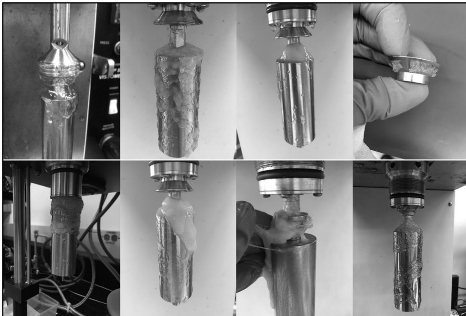
Fig. 5-5 Unbroken polymer residue remaining after various breaker evaluation tests at 300°F (oxidizers and acids), yet they still exhibited low final viscosity (< 50 cp @ 100 s -1 ).
