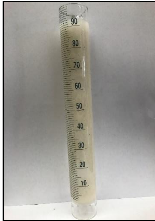
Fig. 2-32 Stable proppant suspension at 40 lb/1,000 gal dual polymer fracturing fluid, 4 gpt crosslinker, pH 5, and 77°F for 24 hours.
