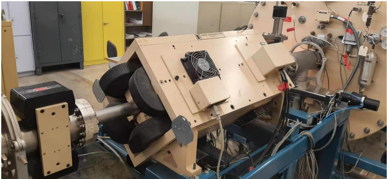
Figure 2.5. Image of quadrupole with its distinctive four poles used for the collimation of the ion beam downstream of the Van-DeGraaf accelerator.
