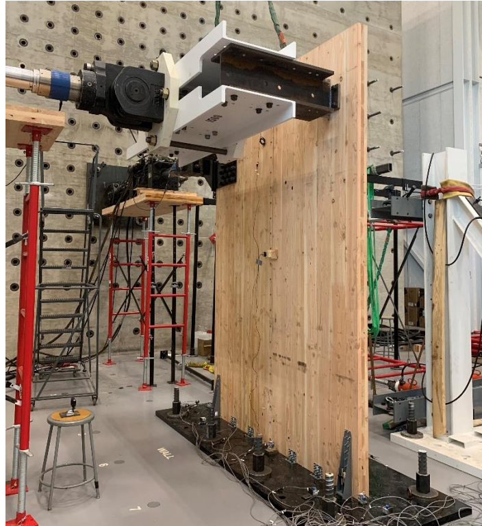
Figure 6.22. Wall-Only Test Setup
