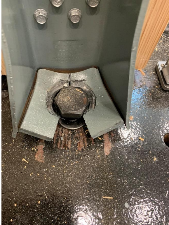
Figure 6.36. Test B2 Hold-down Failure
