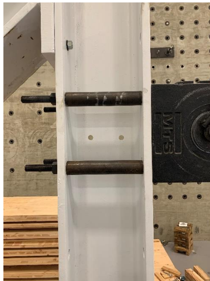
Figure 6.18. Actuator Connection to Reaction Frame
