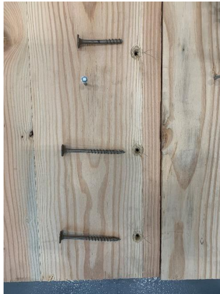
Figure 6.40. Test B2 Panel-to-Panel Connection Failure
