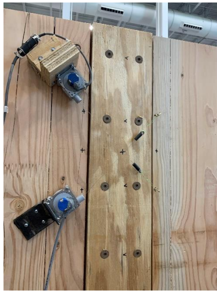
Figure 6.30. String Pots Used to Measure Panel Separation
