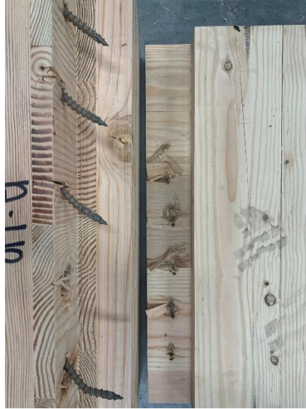
Figure 3.33. Monotonic Fastener Failure
