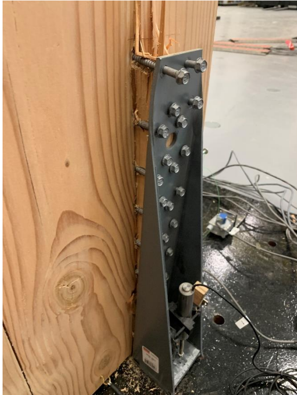
Figure 6.37. Test B4 Hold-down Failure
