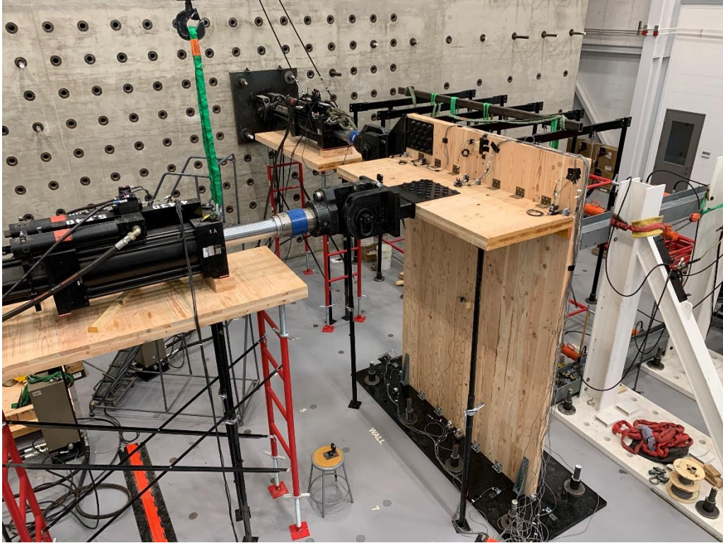
Figure 6.21. Test Setup Including Floor Diaphragm
