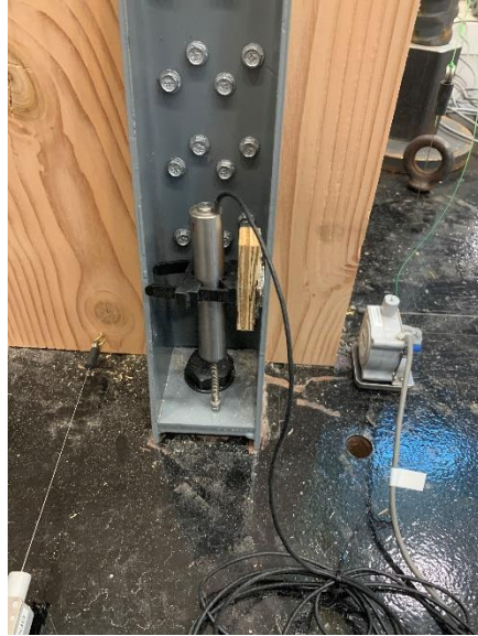
Figure 6.29. LVDT Used to Capture Hold-down Plate Deflection
