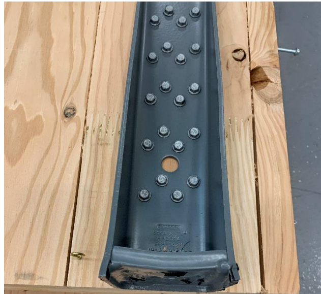
Figure 6.46. Test B6 Damage to Hold-down Connector
