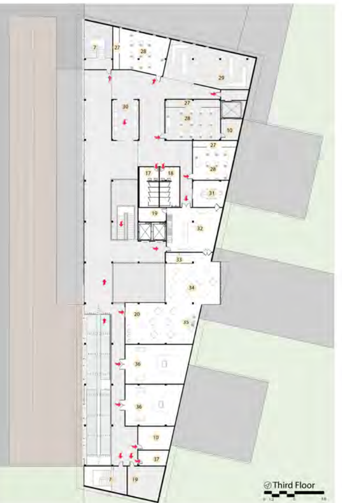
Fig 4.12 Third Floor Column Grid and Circulation
