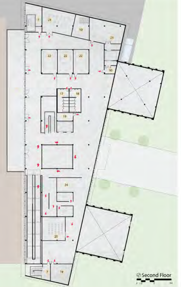
Fig 4.11 Second Floor Column Grid and Circulation
