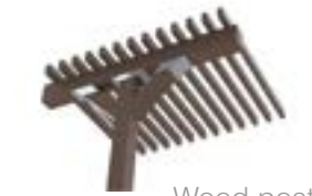
Wood post and beam joint
