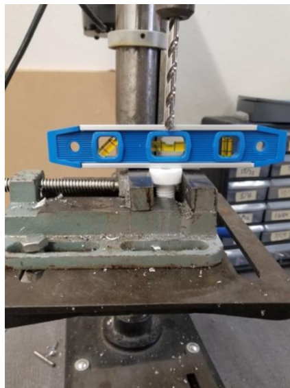
Figure 6.5: Plug Adaptor Leveled Before Drilling
