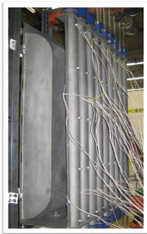
Figure 4.4: Riser Panel with Thermocouples Installed on the Walls and Water Probes
