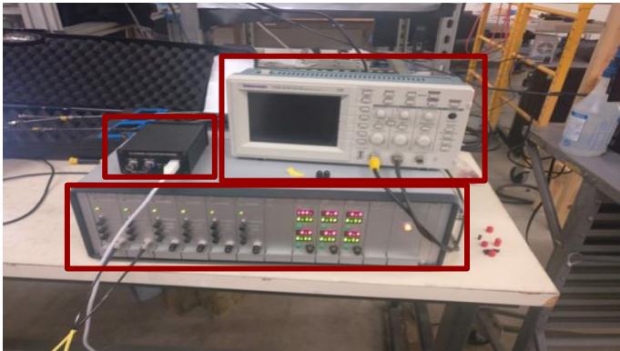
Figure 5.7: Oscilloscope, Acquisition Module, and Opto-Electronic Unit Connected and Operating
