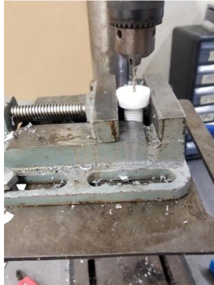
Figure 6.6: Drilling Through the Plug Adaptor with a 1/8 Drill Bit
