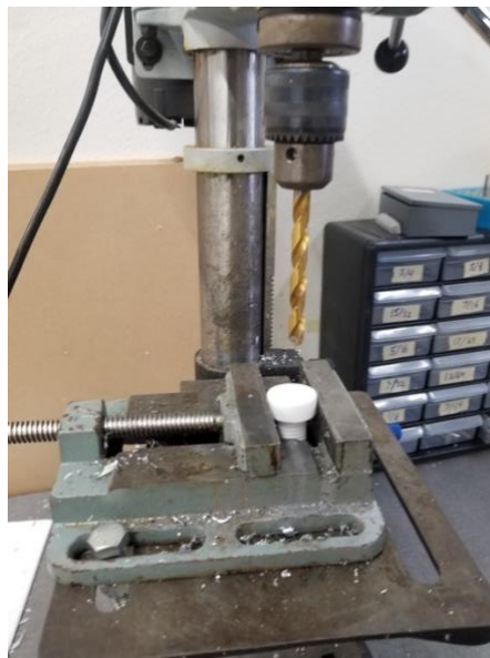
Figure 6.8: Drilling Through the Plug Adaptor with a 3/8 Drill Bit
