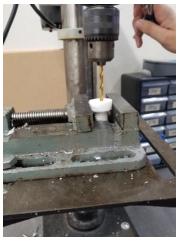
Figure 6.7: Drilling Through the Plug Adaptor with a 3/16 Drill Bit
