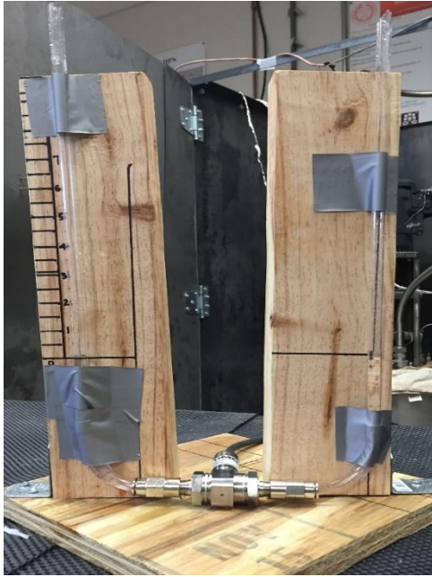
Figure 37. U-tube device used for calibration the pressure transducer before flow experiments (LEFT). The measurement port (Cross union) fixed in the flow apparatus along with connection tubing to Differential Pressure Transducer (DPT) (RIGHT).
