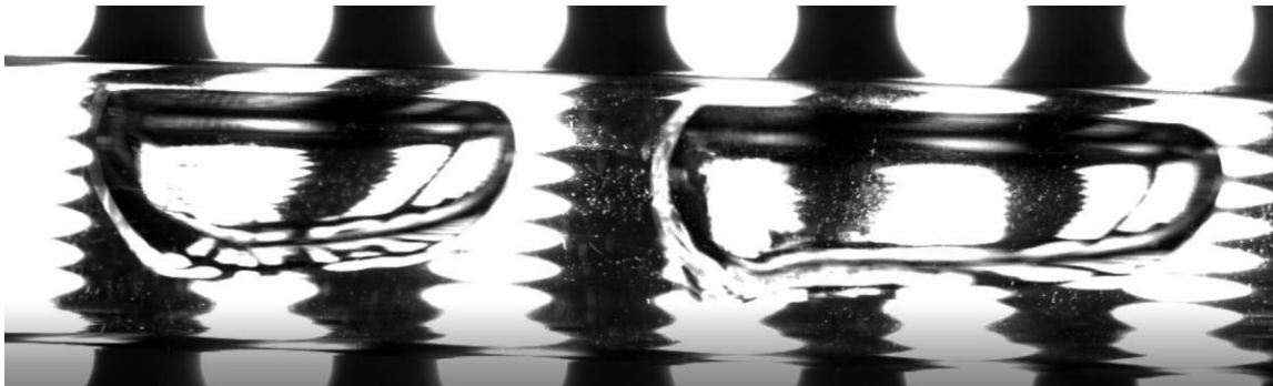
Figure 123. Image of bubble in the flow for DI Water at the end of the test section for a mass flux of 165 [kg/(m 2 s)] at a wall heat flux of 16.9 [kW/(m 2 )]
