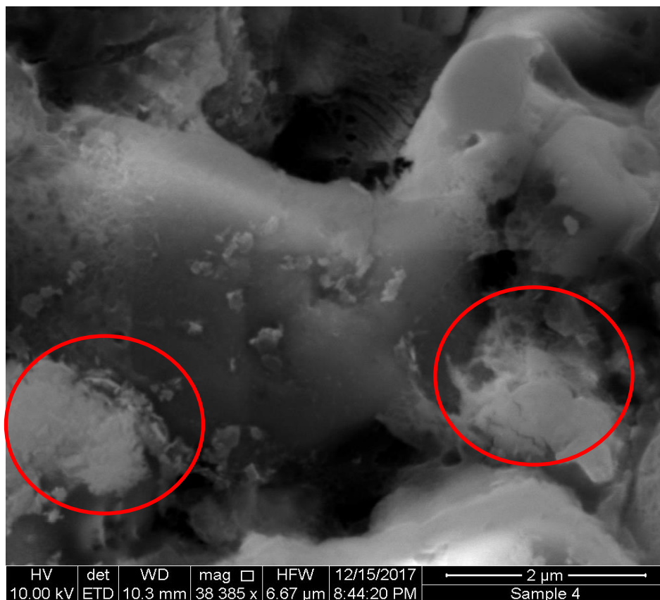
Figure 91. SEM image of ternary nitrate salt e nanofluid sample with 1% target concentration of Alumina generated from thermal decomposition of 6.9% mass fraction of Aluminum nitrate nonahydrate precursor.
