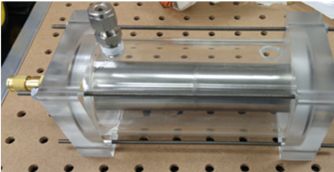
Figure 5.3: Metal hydride pod schematic diagram (top) and image (bottom).
