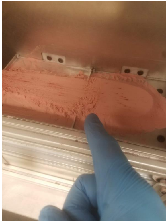
Figure 13: Rut Formed Between Powder Beds
