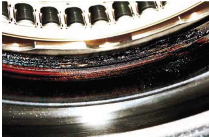
Figure 1 Sample of coke deposits. Reprinted from ExxonMobil [4].
