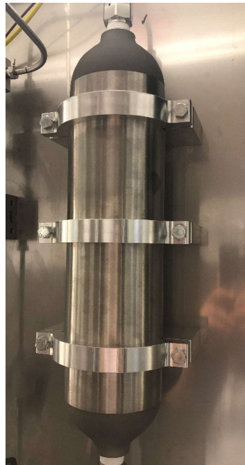
Figure 16 Top reservoir mounted onto the front panel.
