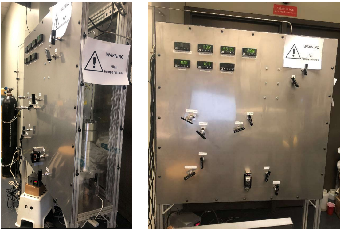
Figure 20 Final test rig with stainless steel front panel and polycarbonate back and side panels.
