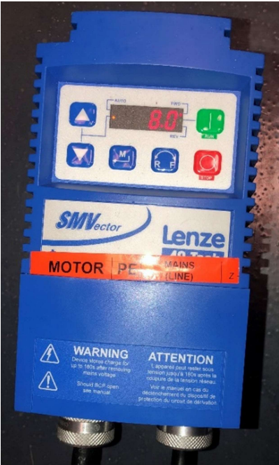
Figure 12 Variable-frequency drive for pump.
