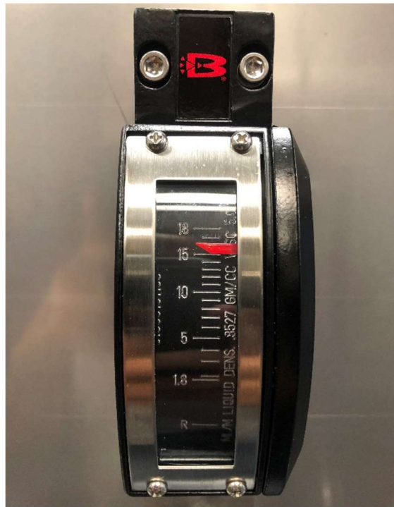
Figure 13 Flow meter mounted to the test rig's front panel.
