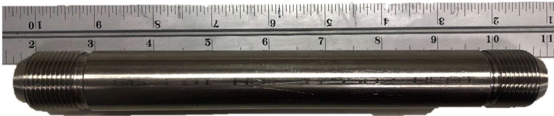
Figure 14 Test section tubing with machined cones and threads.
