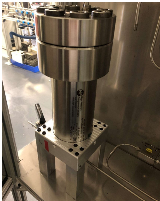
Figure 10 Bottom reservoir mounted on its stand.
