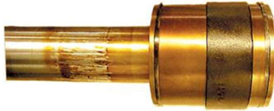
Figure 3 Varnish on an inlet guide vane valve. Reprinted from Fitch and Gebarin [18].
