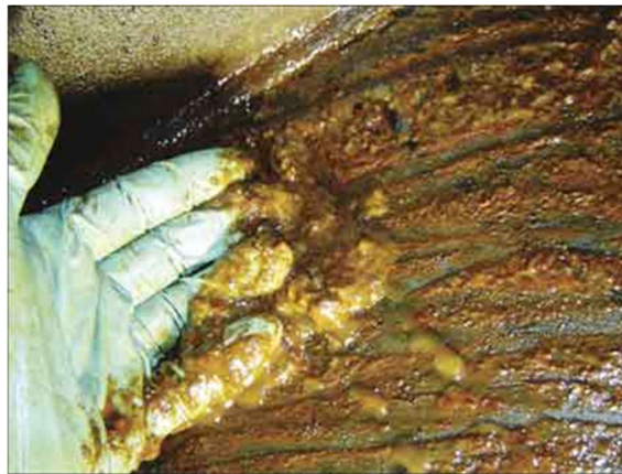
Figure 4 Sludge formed from lubricating oil. Reprinted from Livingstone et al.[23].
