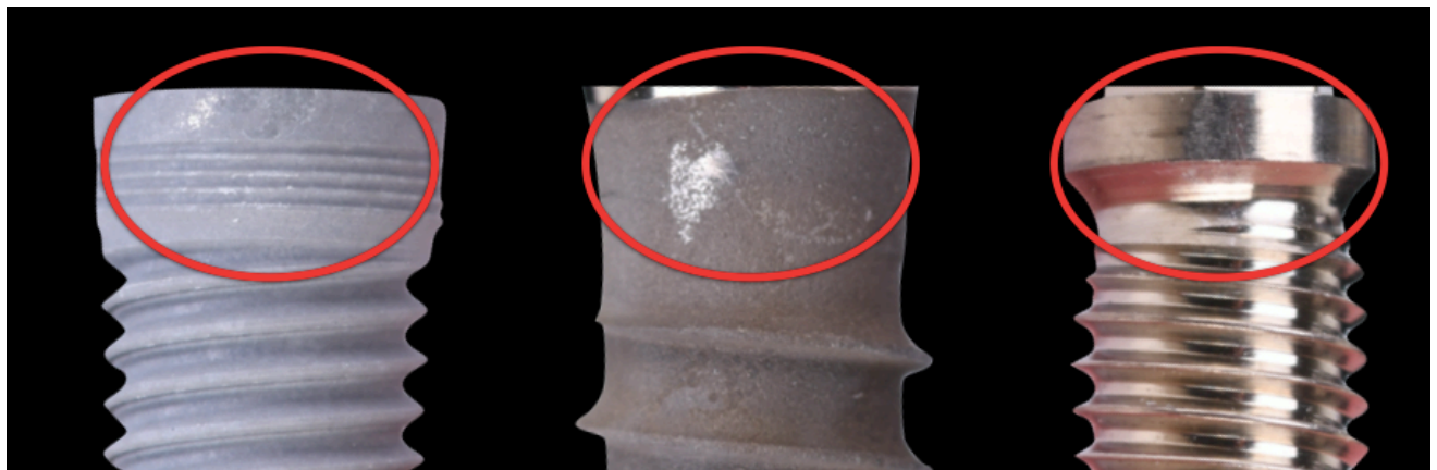
Figure 4. Anodized, SLA, and machined surface implant post instrumentation.
