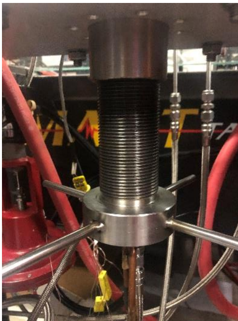
Fig. 18: Burner Vertical Translation Mechanism
