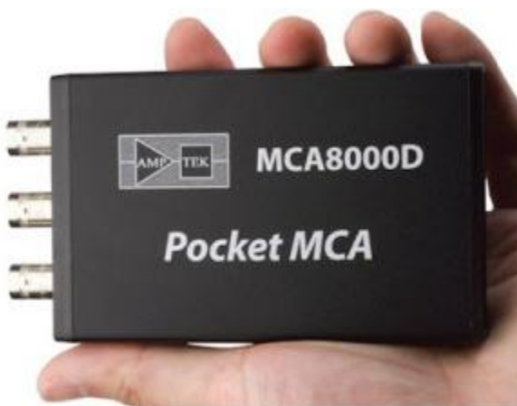
Figure 13. AMPTEK MCA8000D Pocket MCA used in this experiment. Image used with permission from manufacturer. (AMPTEK n.d.).
