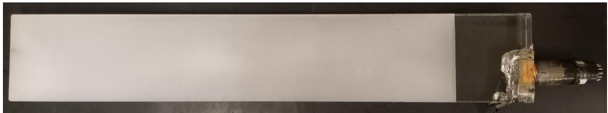
Figure 3. PVT detector exhibiting permanent fogging after extreme temperature and humidity cycles in an environmental chamber. The clear plastic portion of the detector is composed of Polystyrene, usually adhered onto PVT detectors to aid in scintillation light transmission into the photomultiplier tube.
